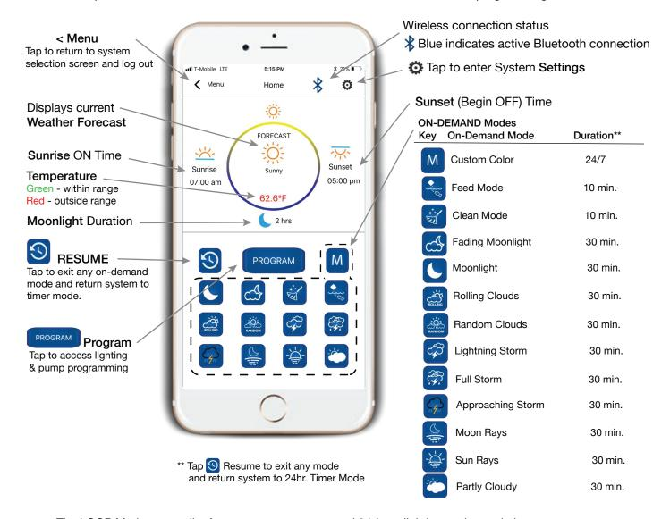
The LOOP Marine controller features a pre-programmed 24-hour lighting cycle to mimic nature.
